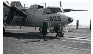
▶ PREPARING FOR TAKE-OFF Deck crew secure a Northrop Grumman E-2C Hawkeye AEW aircraft to a catapult shuttle.
